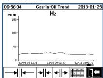
A graph displaying the trend over the time, in this case Hydrogen ( $H_2$ ), is shown.
